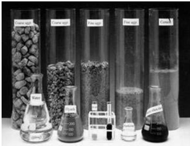
**Figure 23:** A typical mix for a HPC with a maximum water-binder ratio of 0.35. A three-powder binder combination is used, comprising OPC, flyash and silica fume. Such a mix is extremely sensitive to correct execution and curing. All additives and admixtures have to be mixed into the bulk of the concrete, but mostly only needed in the cover zone - A noticeable waste in all aspects. (Photo: N. Thaulow).
